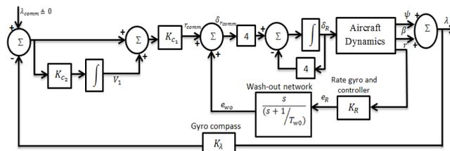
**Fig.12** Heading Control System
