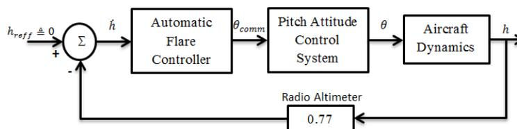
Fig.17 Block Diagram of Automatic Flare Control System
