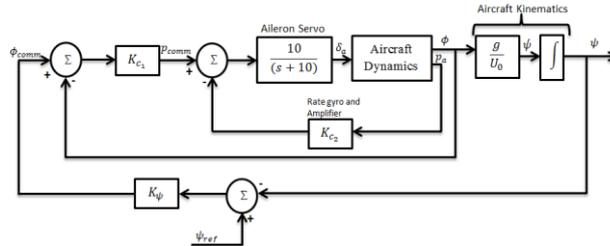
**Fig.10** Direction Control System
