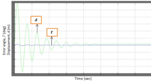
Fig. 15 Response of Glide Path Coupled Control System
