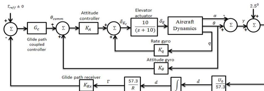
Fig.14 Glide path coupled control system
