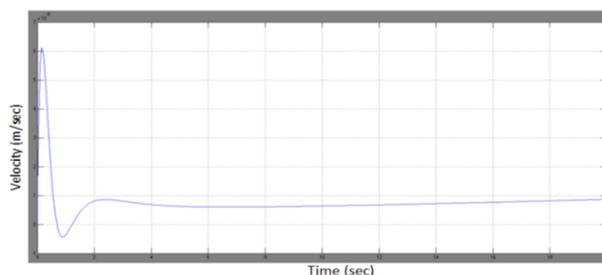
Fig. 9 Response of Mach Hold Control System
