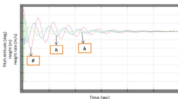
Fig. 18 Response of Automatic Flare Control System
