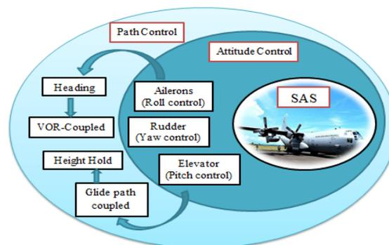
**Fig. 1** Stability augmentation system
