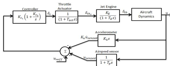
Fig.6 Speed Control System
